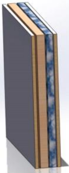
System C. From right to left: sandwich panel; air interspace; cork panel; sandwich panel.
