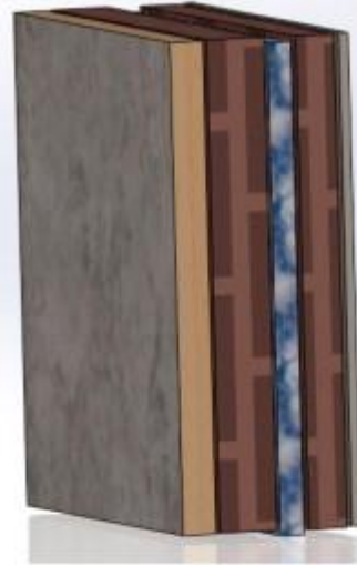
System B. From right to left: cement; perforated brick 8; air interspace; perforated brick 12; bioverd.
