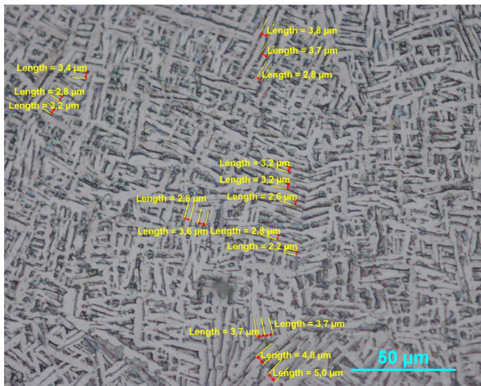
Figure nº 12. Build direction (XY plane). Alpha plates at 500 x of sample 2.
