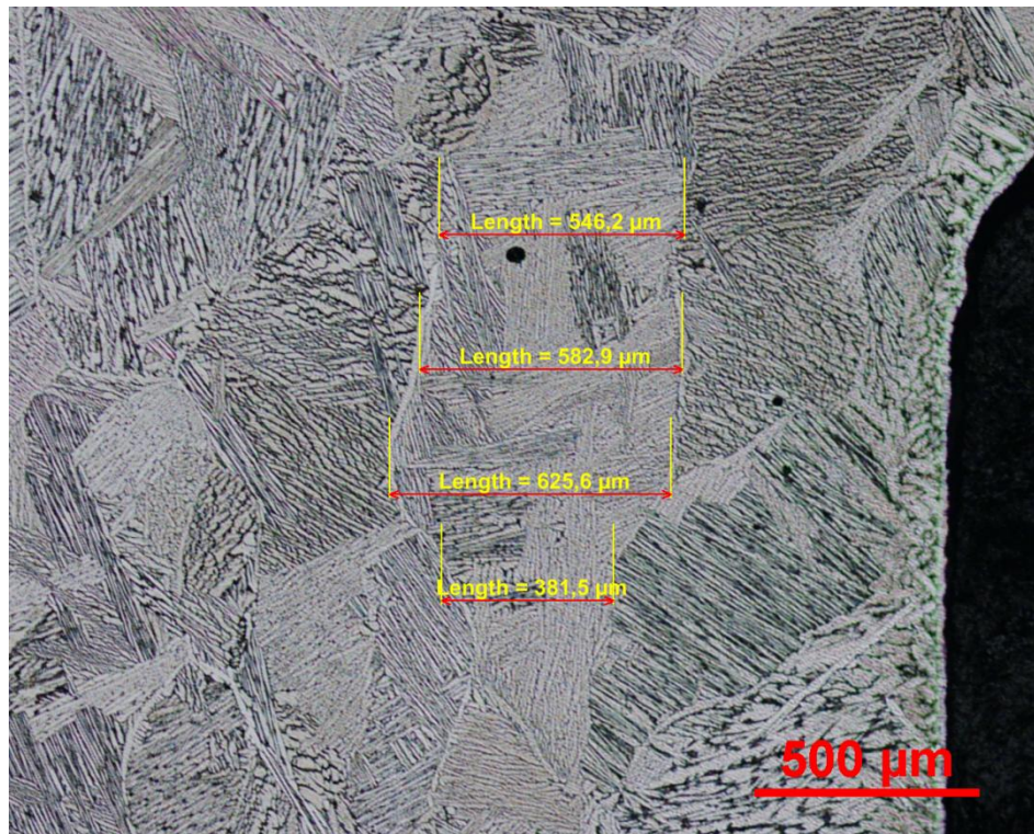
Figure nº 21. Build direction (XZ plane). Grain size at 100x of sample 3.
