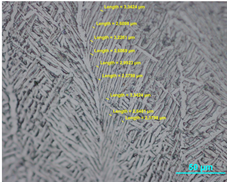
Figure nº 16. Build direction (XZ plane). Alpha plates at 500 x of sample 2.
